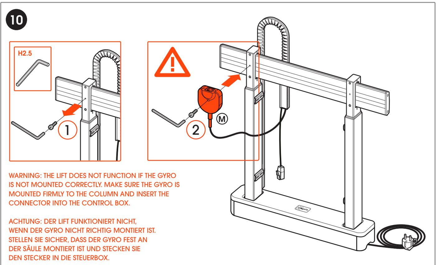
**WARNING: THE LIFT DOES NOT FUNCTION IF THE GYRO IS NOT MOUNTED CORRECTLY. MAKE SURE THE GYRO IS MOUNTED FIRMLY TO THE COLUMN AND INSERT THE CONNECTOR INTO THE CONTROL BOX.**
