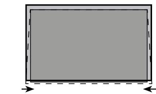
Should the two rear levelling feet have reached their max. height and cannot be turned out more, then you can try turning in the two front levelling feet instead.
