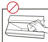
The lens must not be touched directly or wiped with a cleaning cloth. Doing so may damage the lens coating, which would negatively affect the image quality.
