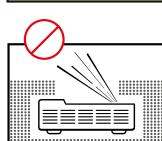
The Laser TV must not be set up in an enclosed space with limited ventilation. Doing so would cause the device to overheat.
