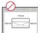
The recommended distances (see illustration) must be adhered to in order to ensure sufficient ventilation for the device.
