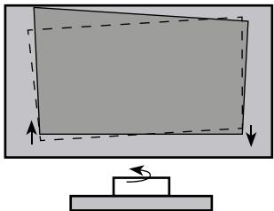
The lower edge of the image is higher on the left and lower on the right
