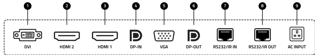
① DVI - ② HDMI2 - ③ HDMI1 - ④ DP-IN - ⑤ VGA - ⑥ DP-OUT - ⑦ RS232(RJ45)/IR IN - ⑧ RS232(RJ45)/IR OUT - ⑨ AC INPUT
