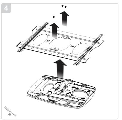
To ease the installation process you have the option to remove the wide front plate and mounting brackets by simply removing the three M5 x 10mm flat head screws, holding the plate assembly to the swing out arm assembly and setting them aside.
