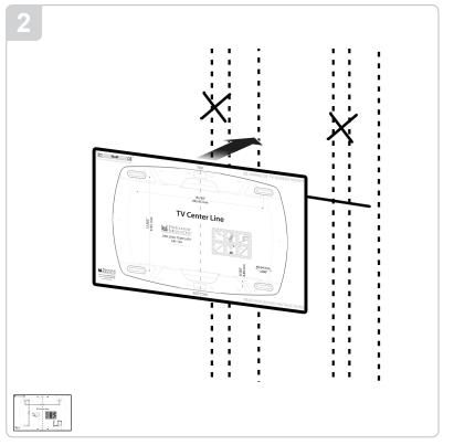
Take the thick cardboard mounting template supplied and place the it over the mounting studs with the screen center facing up. Confirm that the template is level horizontally and that the wall place outline is to the center of your desired height.
