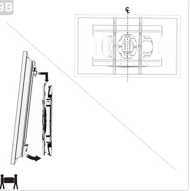
With the upper and lower security screws loosened on each bracket (two people recommended) raise the display and place the top hook of the bracket over the receiver plate on the wall mount. Allow the lower end of the bracket to lay flat against the mating plate on the mount.
