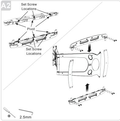
Remove the plastic hole covers from the upper and lower plates. Loosen the (2) set screws on the plate using the 2.5mm allen key supplied. Reposition the upper and lower pivot rods to mate to either the center or right side pivot receiver holes, push the upper and lower plate fully on to the rods, and re-tighten the set screws. Reinstall the side plate with the eight flat head screws and confirm they are secure. Reinstall the round plastic hole covers.
