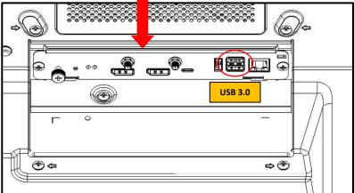
Connect the Huddly camera: Connect the 2 m USB cable supplied with the Huddly camera from USB-C of the camera to one of the USB 3.0 ports of the OPS slot-in PC.
