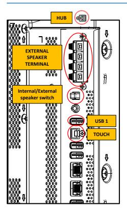
**4. Enable touch**: When used with an OPS slot-in PC no external USB cable is needed to activate touch.
