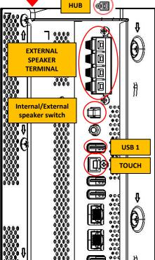
1. Enable the USB hub: Use the short 10 cm USB cable supplied with the monitor. Connect USB cable from USB Type-B input marked with "Hub" (located above external speaker terminals) to USB Type-A input marked with "USB 1" on the side of the monitor. The red LED on the USB hub will light up.
